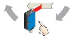
Press teach-in button > 1 s when transmitted light is red = tolerance coarse.
